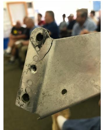
Tom showed the membership some of the corrosion and cracks found during a more detailed inspection of several aircrafts. He included the outboard rib of a P28 with extensive corrosion. It weakens the structure of the leading edge, and is indicative of water leaking under the tips. This probably would have eventually become a hole in the wing skin. Catching it early made it only a \$600 repair compared to a several thousand dollar repair for the leading-edge and skin.
