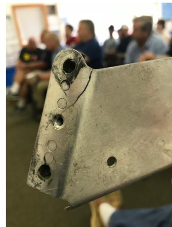
Tom showed the membership some of the corrosion and cracks found during a more detailed inspection of several aircrafts. He included the outboard rib of a P28 with extensive corrosion. It weakens the structure of the leading edge, and is indicative of water leaking under the tips. This probably would have eventually become a hole in the wing skin. Catching it early made it only a \$600 repair compared to a several thousand dollar repair for the leading-edge and skin.
