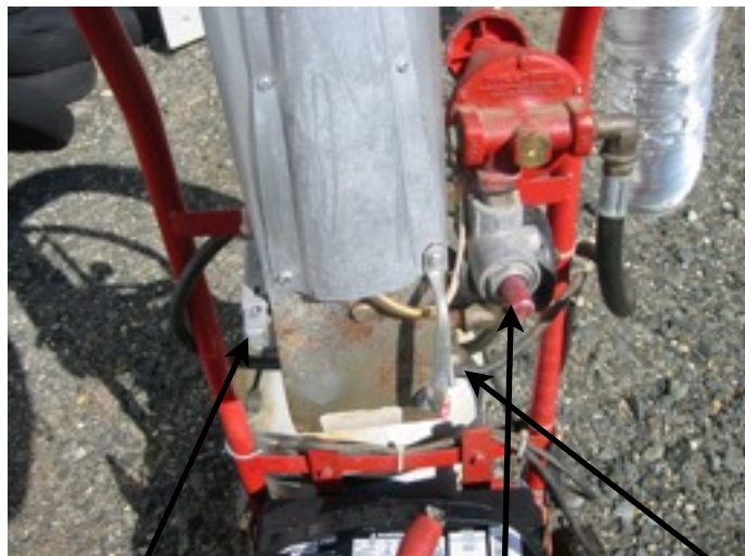
Press the igniter (left) and the fuel supply button (right)
