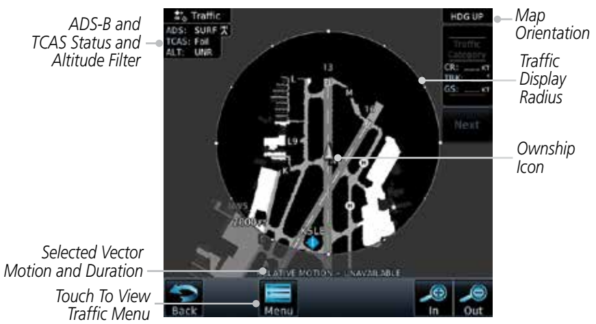
Figure 4-3 SURF Display with the GTN 7XX
