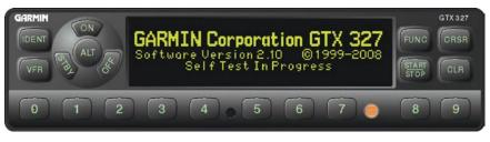
The GTX 327 transponder is powered on by pressing the **STBY**, **ALT**, or **ON** keys, or by a remote avionics master switch (if applicable). After power on, a start-up page is displayed while the unit performs a self test. If the unit detects an internal failure, the screen displays SELF TEST FAILED.
