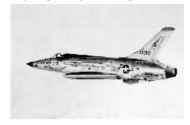
The Republic F-105 Thunderchief was the first supersonic tactical fighter-bomber developed from scratch. Apart from being the biggest single seat, single-engine combat aircraft in history, the F-105 was notable for its large internal bomb bay and unique swept-forward engine inlets in the wing roots. The wing was highly swept and incorporated low-speed ailerons and high-speed spoilers for lateral control, and a droop-snoot leading edge.
